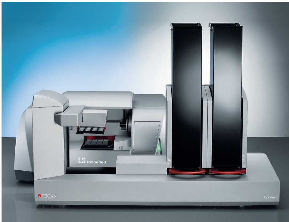
Fig. 1: Tecan Connect™ (in front) in combination with Tecan LS Reloaded (background) Tecan Connect: left: tower with gripper; right: two magazines to store microplates Photo courtesy of Tecan Group Ltd.
